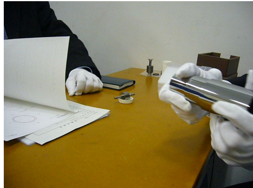
Hokkai M.I.C. Cylinders with 2 micron clearance
